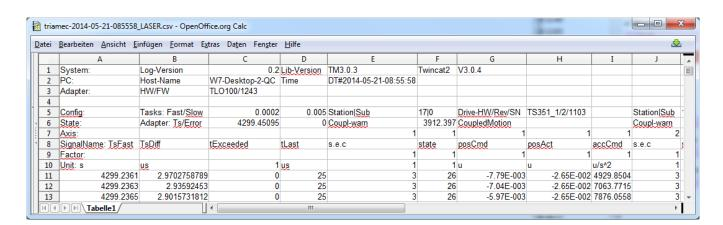
Column G are commanded positions at the input TL\_AxisFast::PosIn in PLC units. Please note the factor 1000 in cell G9, which is TL\_AxisSlow::Config.GearFactor. This means PLC positions are divided by 1000 before being sent to the axis.
