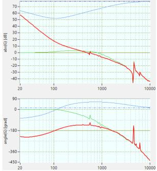
Figure 6: Bode plot of the tuned linear axis.
