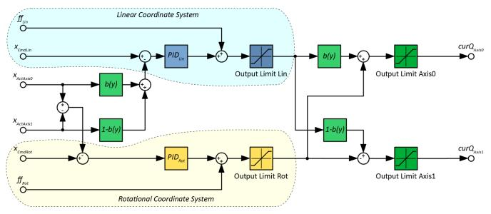
Figure 2: Structure of decoupled gantry controller.
