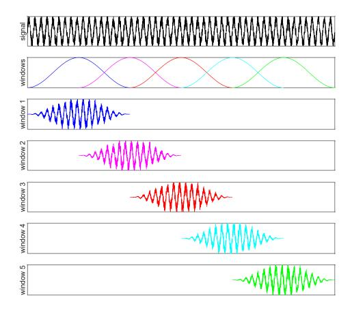
The window function is calculated every 10kHz. The FF has a 2048 tap window with an overlap of 1048 = 2048 - 1000 taps.
