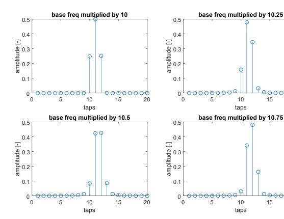
Figure 1: Base frequency multiples between 10 and 11
