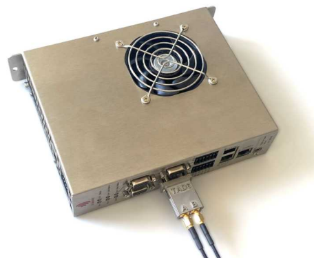
Figure 3: TAD6 mounted on Axis 0 of a TSD80
